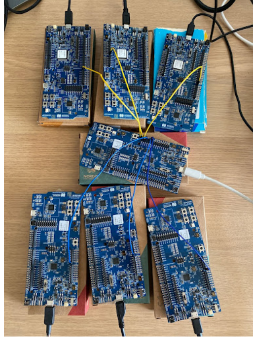
Figure 8: Shown in figure: 3 nRF52840dk boards and 3 nRF5340's all connected through pins and powered with a USB hub. The two boards appearance is very similar.
